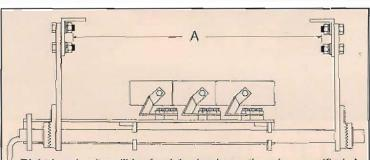
Right hand units will be furnished unless otherwise specified. A right hand unit will have the adjusting handle on the right hand side when facing the direction of travel of the load on the conveyor belt. Dimension "A" adjusts to fit conveyor frame with a minimum of 5" greater than the belt width and a maximum of 21" greater than the belt width.
